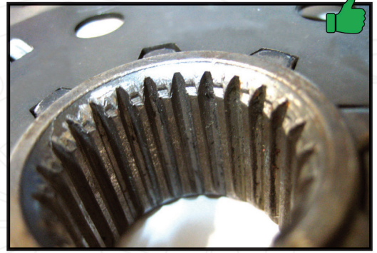
Example of PERFECT AMOUNT OF GREASE . As you can see, it is barely visible to the naked eye and acts as more of a lubricant.
