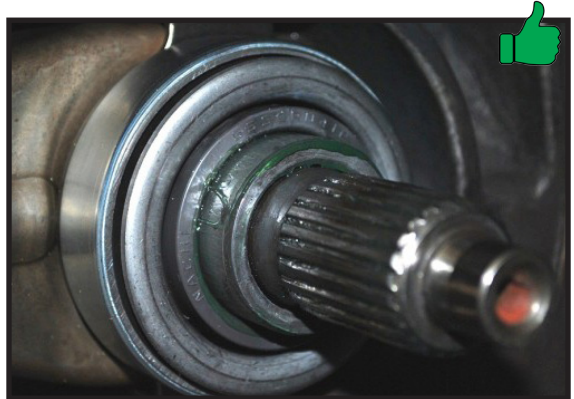
Example of PERFECT AMOUNT OF GREASE on the input shaft. As you can see it is barely visible to the naked eye and acts as more of a lubricant.
