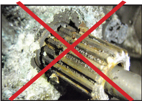
Example of TOO MUCH GREASE on input shaft, which causes grease to spray all over the disc and ruin the disc material or pads.
