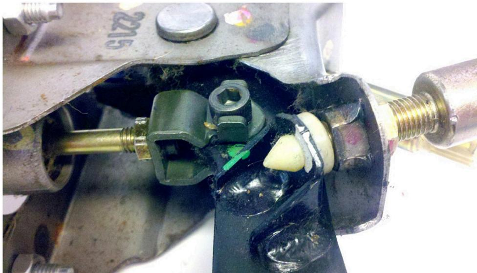
10. Loosen the lock nut on the upper switch and back the switch out until the threaded portion of the switch is flush with the bracket.
